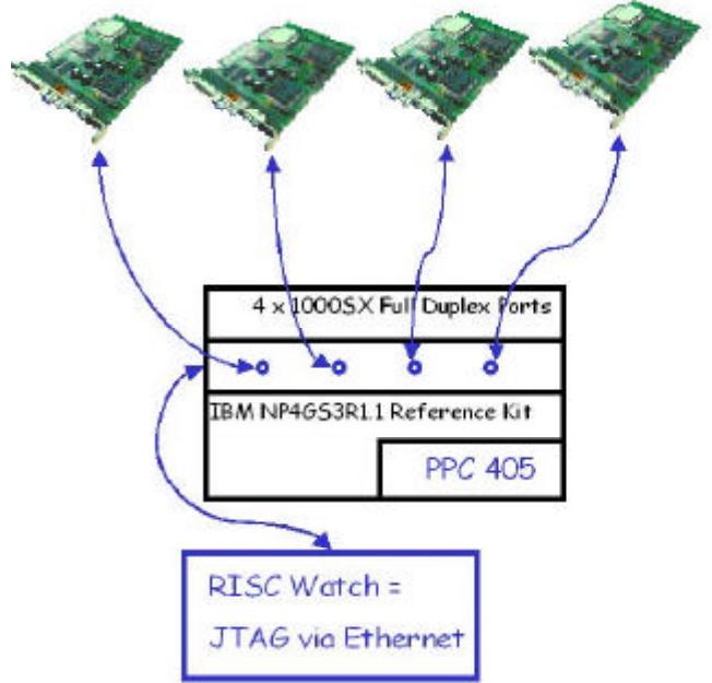
Figure 7: Test-setup for the NP4GS3 reference kit. The data are fed and read back using Tigon 2 based Gigabit Ethernet NICs. Download of NP software and monitoring of the NP is done via JTAG using the RISCWatch probe
