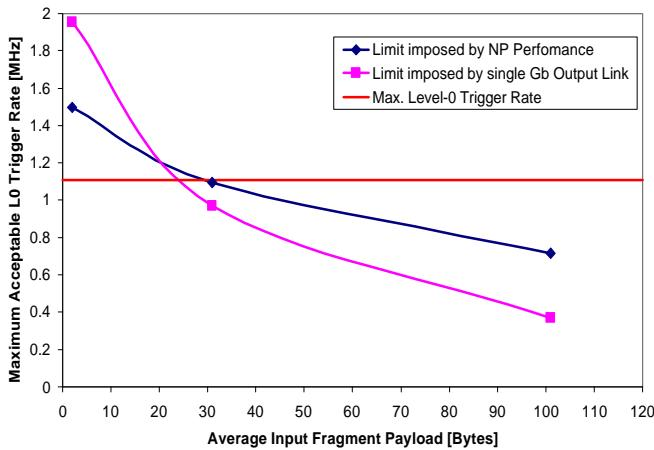
Figure 5: Performance of Ingress event-building from simulation as a function of the average incoming packet size. The straight line shows the fixed level 1 trigger rate of 1.1 MHz. The limitation on performance comes from the output link bandwidth only.
