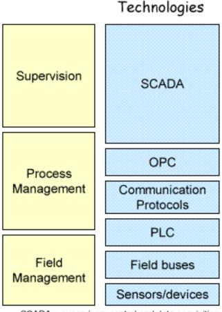
SCADA = supervisory control and data acquisition OPC = OLE for process control PLC = Programmable logic controller Eield buses = CAN, ProfiBus, WorldFip, ...
