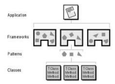
Each design pattern is a micro-architecture for a recurring element. Patterns can represent generic software elements, or elements that are particular to a problem domain. When you design a framework, look for recurring patterns that can be applied to other problems.
