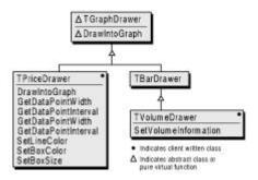
TPriceDrawer charts stock prices, displaying high, low, and close prices for a particular stock. This class is derived directly from TGraphDrawer and from MStockHolder, which holds a collection of daily stock data. TPriceDrawer overrides TGraphDrawer::DrawIntoGraph, and provides functions for manipulating the data points and attributes.
