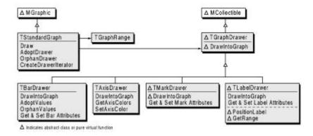
To use the framework, a client constructs the necessary drawers and a standard graph. When the client calls TStandardGraph::Draw, DrawIntoGraph is called for each drawer and the graph and all its elements are drawn. To change the appearance of the graph, clients can call functions such as TAxisDrawer::SetAxisColor.
