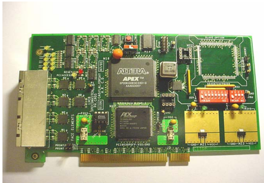
Figure 11 : Photograph of a SPECS Master Prototype board
