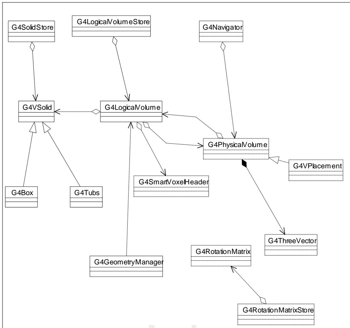
Figure 8: GEANT4 geometry data model
