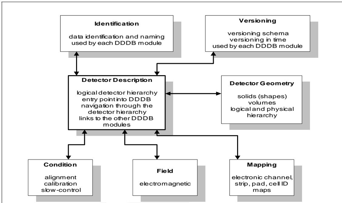
Figure 1: Detector data model schema
