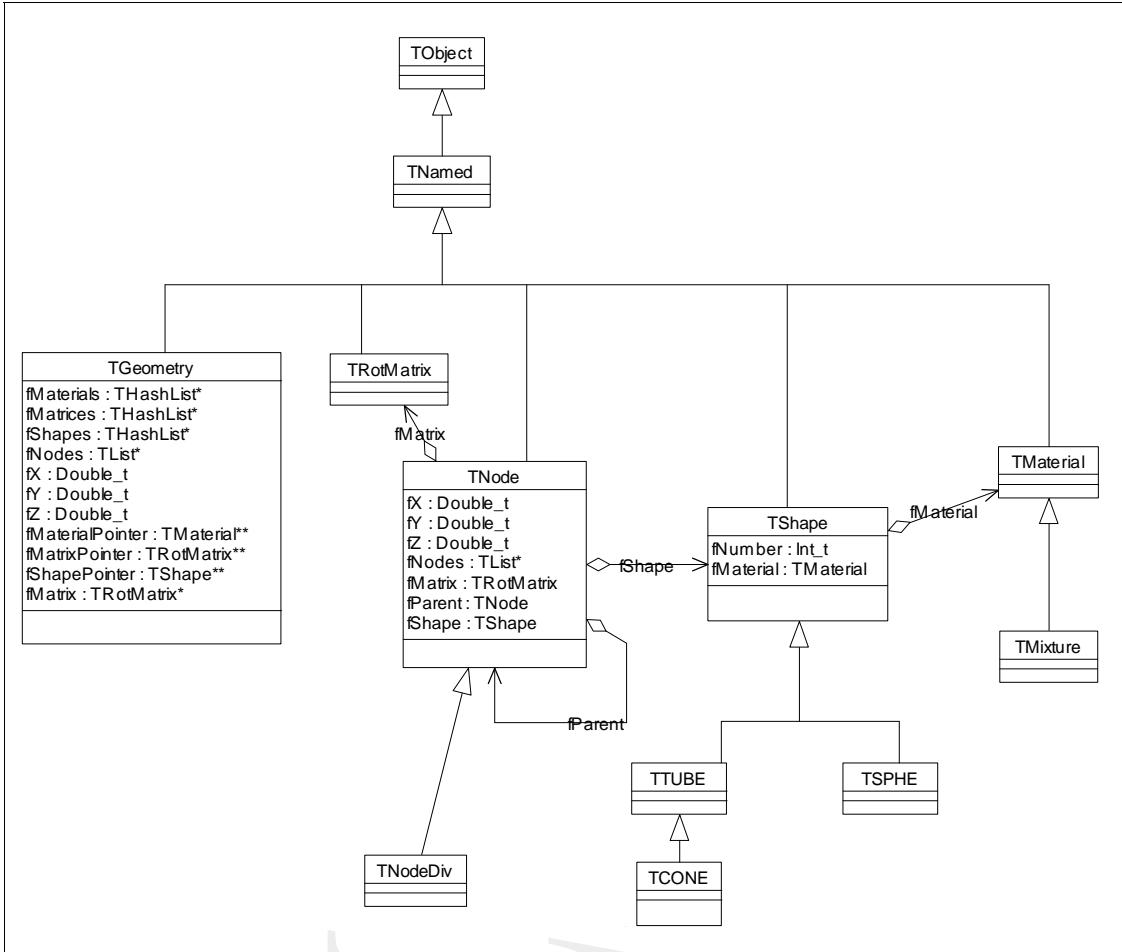
**Figure 9:** ROOT geometry data model.
