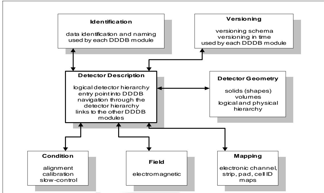
**Figure 1:** Detector data model schema
