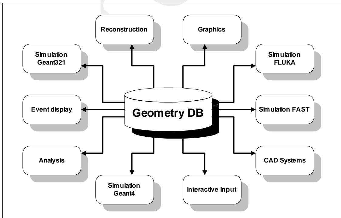
Figure 7: ALICE geometry database system overview
