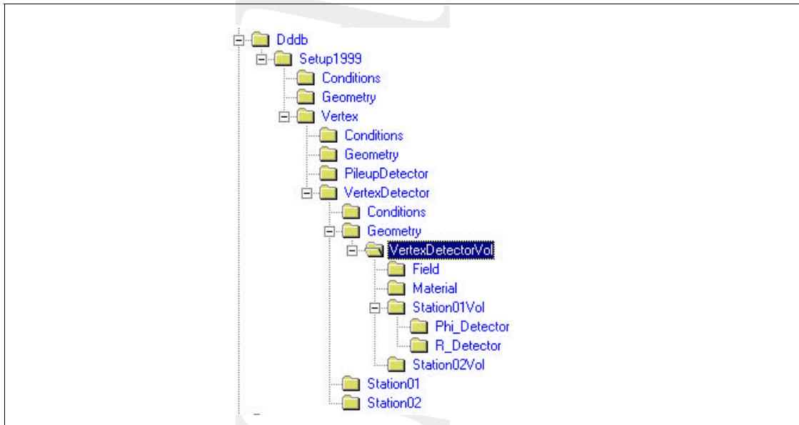
**Figure 3:** Detector description hierarchy in the transient detector data store
