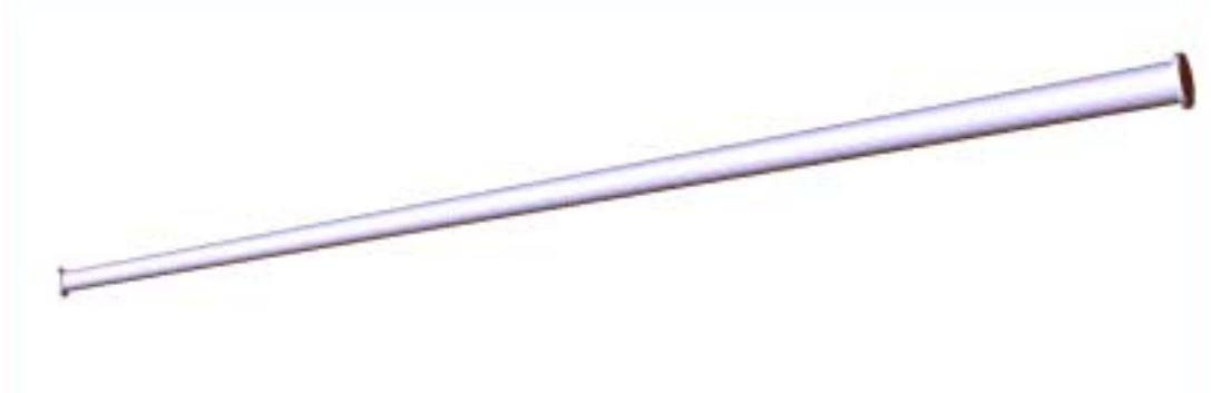
Figure 4: Beam Pipe Sections 4 starts at z \sim 3.2\text{m} , length \sim 3.9\text{m}
