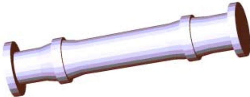
Figure 3: Beam Pipe Section 3 starts at z \sim 2.8\text{m} , length \sim 0.4\text{m} .
