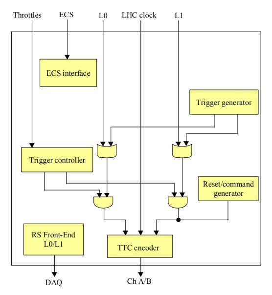
Figure 2 Block diagram of the Readout Supervisor
