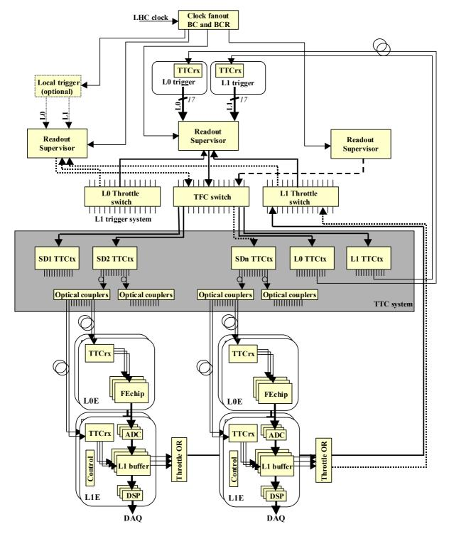
Figure 1: General Architecture of the Timing and Fast Control system
