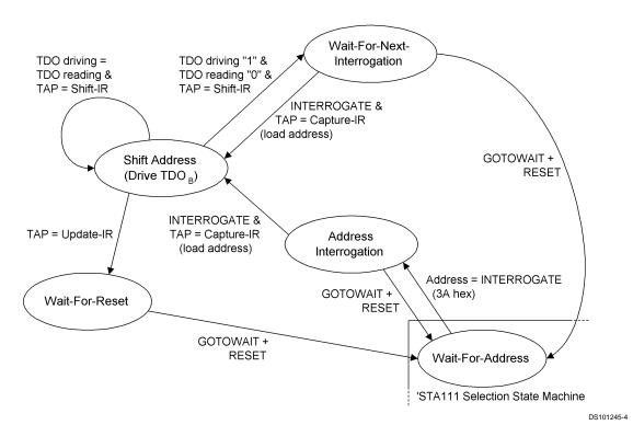
FIGURE 13. Address Interrogation State Machine
