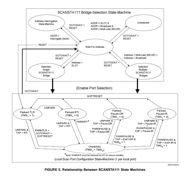
Following a hardware reset, the TAP controller statemachine is in the *Test-Logic-Reset* (TLR) state; the 'STA111selection state-machine is in the *Wait-For-Address* state; and each of the three port-selection state-machines is in the *Parked-TLR* state. The 'STA111 is then ready to receive Level-1 protocol, followed by Level-2 protocol.
